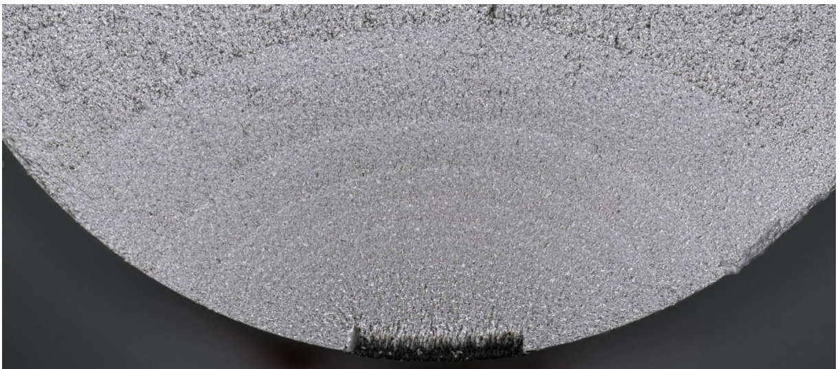
Figure 3.12: Crack surface overload
