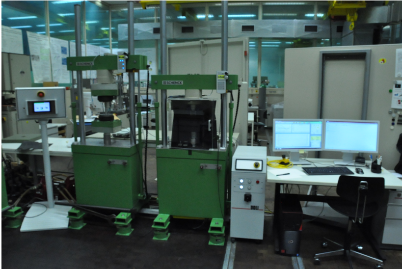
Figure 3.9: Schenck testing machine and DOLI Elettronic system
