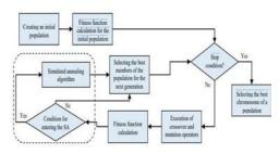
Fig :6 A model of the combination of a genetic algorithm and a simulated annealing algorithm
