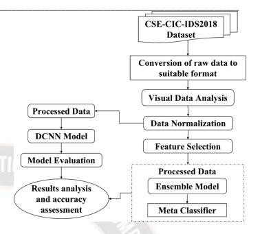
Figure 1. The workflow of the proposed methodology.
