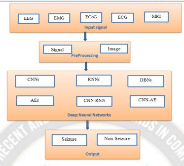
Fig.2. Block Diagram of Deep Learning Based System
