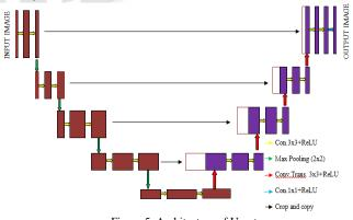
Figure 5. Architecture of U-net
