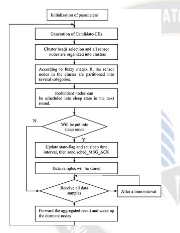
Figure 1. Flow of a typical sleep scheduling energy aware routing model
