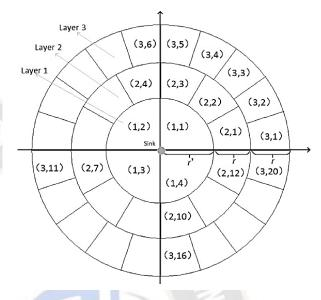
Figure 3. Fan Shaped Clusters for all 'Wake Up' nodes
