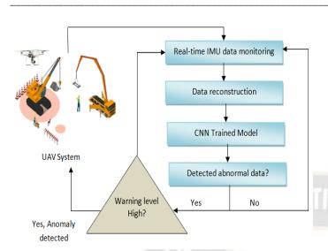
Figure 5: System for Detecting UAV Anomalies
