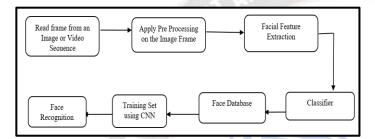
Figure 1. Basic Block Diagram for Face Recognition
