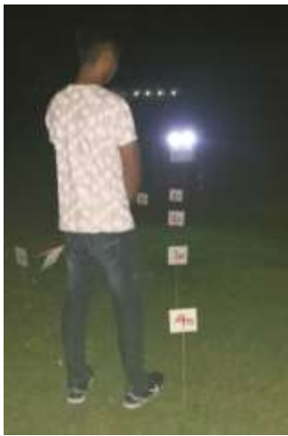
Step 9. Evaluation of lights activation from 1 meter to 7 meters within an angle of 60 degrees right
