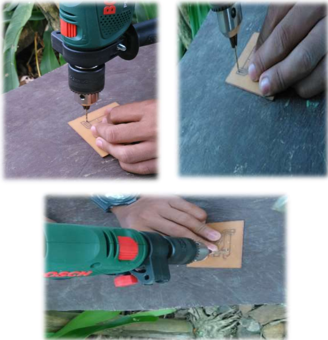
Step 4. Boring holes to the PCB based to the circuit diagram
