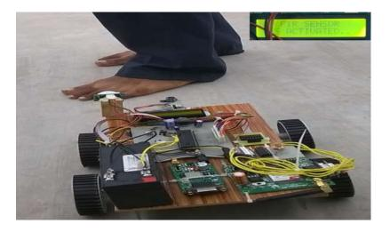
Fig. 8. Human Detector Robot detecting Human with PIR sensor
