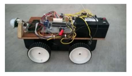
Fig. 5. Prototype of human detection ROBOT
