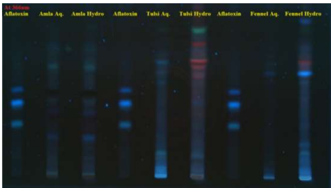
Fig. no. 2: Spots of Aflatoxin and plant extracts on TLC plate at 366nm
