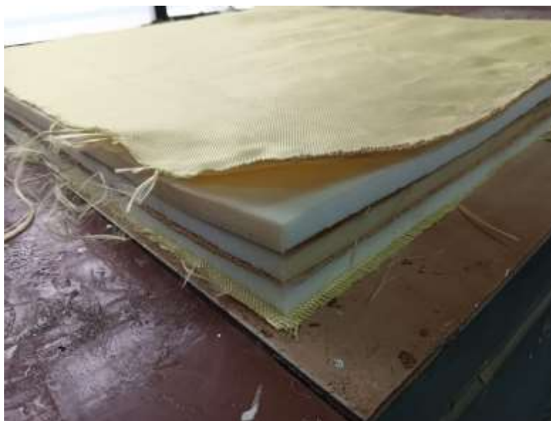
Figure 1. Photograph of impregnated and cured sandwich composite
