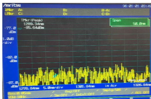
Figure 31: The optical spectrum between 1276 nm – 1326 nm, before the insertion of the classical channels
