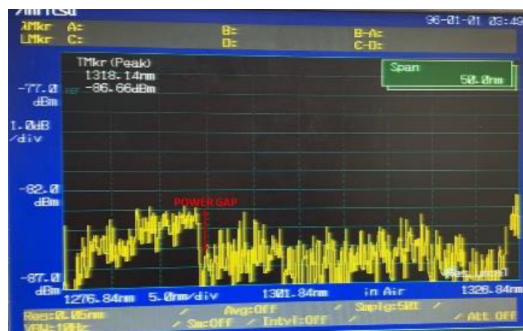
Figure 36: The power gap in the optical spectrum between 1276 nm – 1326 nm
