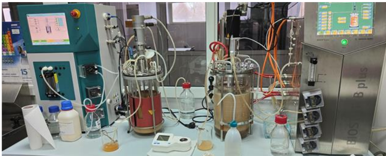
Figure 1 Biostat B+ and Applikon bio - biotechnological process for obtaining wine yeast biomass
