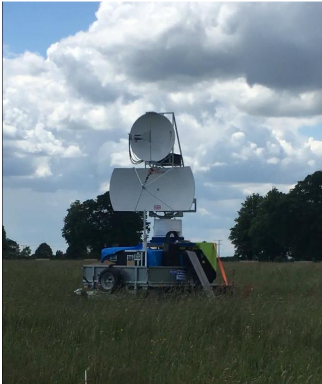
Figure 1.1.5: Scanning harmonic radar from Rothamsted Research, Hertfordshire, UK. Photo credit: Thomas R. Oliver.
