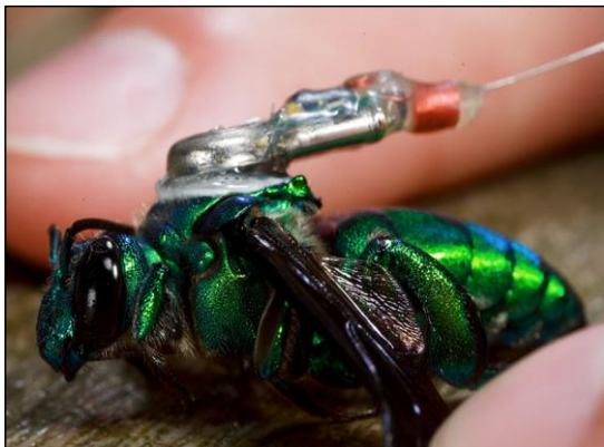
Figure 1.1.1: Attachment of a micro-radio transmitter (300mg) to a male orchid bee Exaerete frontalis . (Wikelski et al., 2010).
