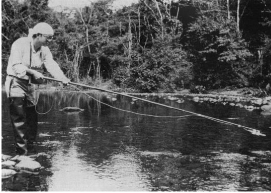
Figure 1.1.2: Position determination of a radio-tagged larva using a small loop antenna equipped at the tip of a rod. This figure has been adopted from (Hayashi and Nakane, 1988) with permission from the publisher.
