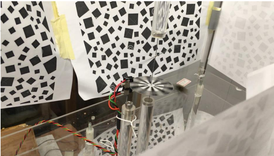
Figure 2.2.4: The flight mill apparatus with bumblebee worker mid-flight. Screens surrounding the mill provide optical flow for the attached bumblebee.
