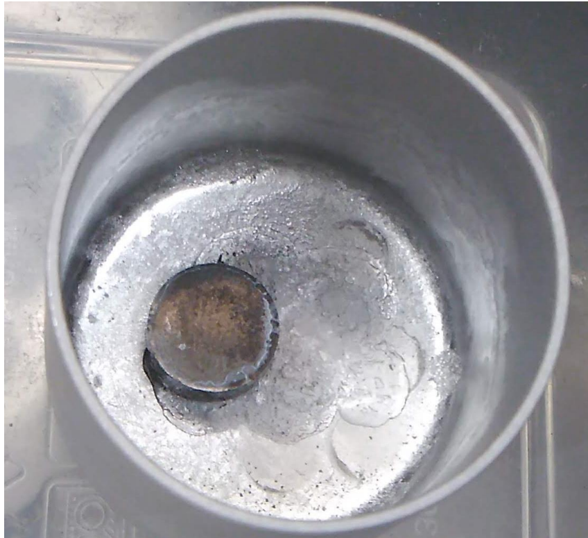
Figure 4.9: Typical sample of UB_2 with impurities of UO_2 .
