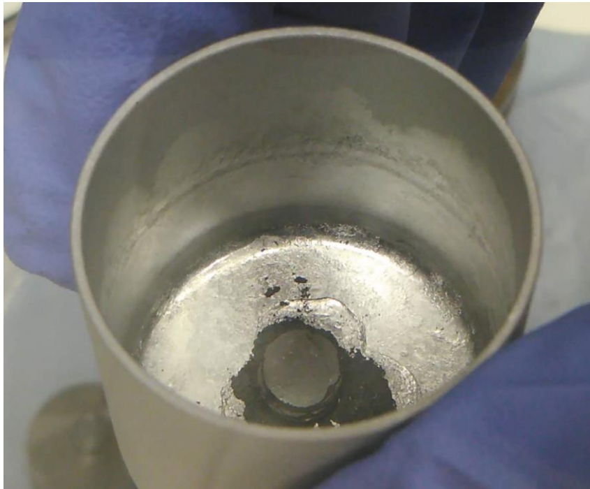
Figure 4.8: Typical sample of UB_2 with high purity.
