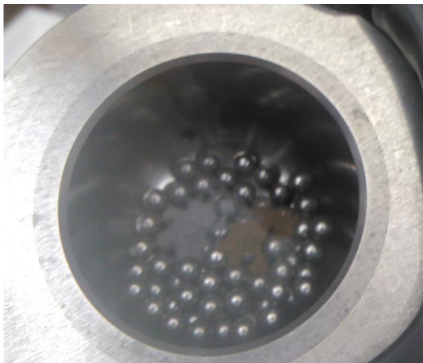
Figure 4.10: UB_4 (left, grey) and UO_2 (right, brick red) in the jar of the ball mill prior to mixing
