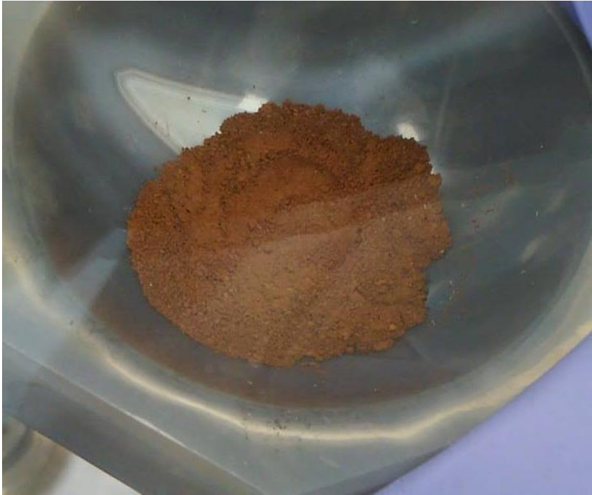
Figure 3.10: \text{UO}_{2+x} prepared from the hydrogen reduction of \text{U}_3\text{O}_8 .
