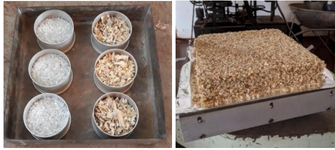
Fig. 1 (a) PET flakes and Pinus particles (b) Particle mattress before pressing
