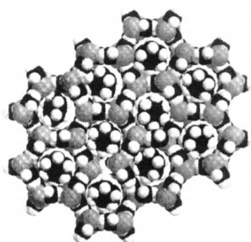
Figure 1.43: Thiourea-cyclohexane inclusion complex at ambient temperature; ten complete tunnels can be seen in which the cyclohexane molecules reside 84
