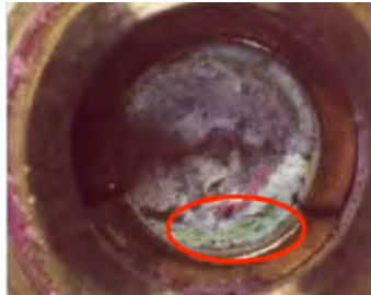
A photo from the Dutch Safety Board accident investigation showing green copper azide crystals (circled) inside the casing of an M-6 mortar bomb fuze. The formation of this sensitive compound is believed to have caused a fatal accident in 2017, and could become a hazard in many types of ammunition as it ages.
