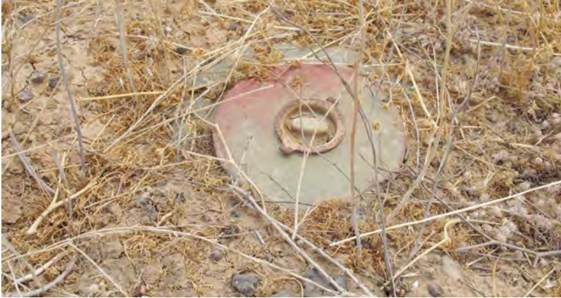
A United States M15 anti-tank mine, encountered in 2010 in a minefield on the Jordanian border with Syria. Disarming this mine should be a simple matter of unscrewing the central plug and removing the fuze; however, the plug is firmly rusted into place. This is an example of ageing preventing a render-safe procedure, leaving demolition as the only practical disposal option. Image: Fenix Insight Ltd.
