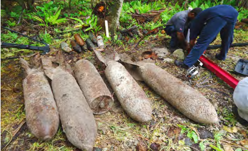
Recovery of Japanese bombs from a buried stockpile. These Type 3 No25 Mk8 Mod1 – 7 bombs are unfuzed, with just a blanking plug fitted into the fuze wells. The absence of a fuze and primary explosive reduces the risk significantly. While a degree of corrosion can be seen, the resilience of the thick cased munitions is evident.
