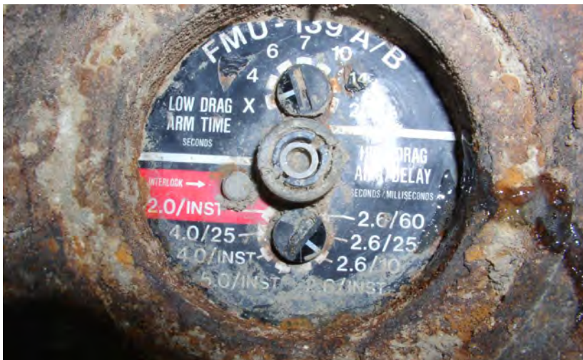
An FMU 139 A/B electro-mechanical fuze in the tail of a MK-83 aircraft bomb in Iraq. The fuze contains capacitors charged from the employing aircraft prior to being dropped. The charge has long since dissipated. Image: Roly Evans.
