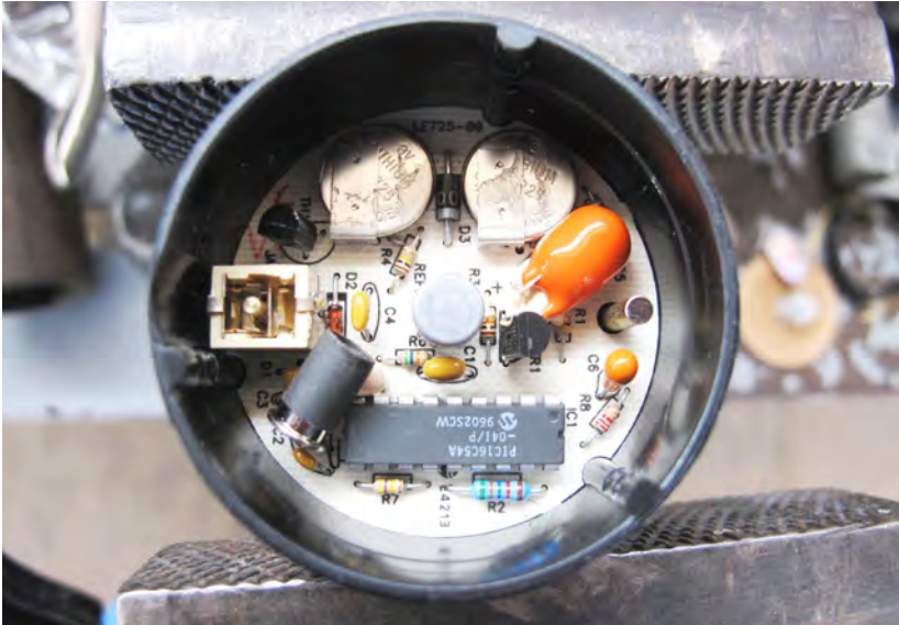
The electronic fuze of a Spanish SNA submunition is powered by two lithium batteries. These batteries are isolated from the circuit until the weapon is deployed. Image: Fenix Insight Ltd.
