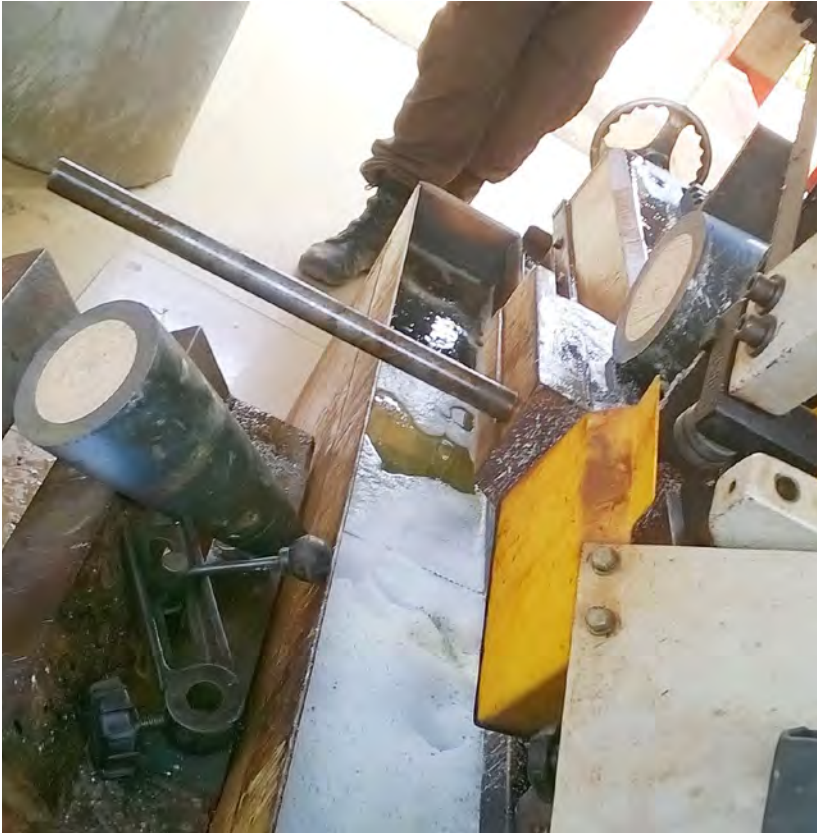
A cut on a Russian 152mm OF-540 high explosive artillery projectile at the Golden West Humanitarian Foundation (GWHF) specialist processing facility in Cambodia. The projectile casing and pressed TNT fill are in good condition and have not been subject to significant ageing in the environment. Image: Roly Evans.
