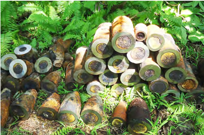
Projectiles that have been cut and inspected await final disposal. Image: Len Austin.
