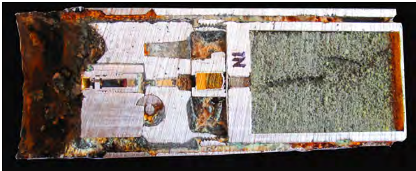
The sectioned body of a Vietnam-era US M904 bomb fuze, recovered in Cambodia. The components of the explosive train are clearly visible running horizontally through the centre of the fuze. Their alignment shows that this section of the fuze was correctly armed. For some reason the striker has not initiated the in line explosive train. The primary explosive may still be viable, as it is well protected by the fuze casing, but the pyrotechnic elements of the explosive train are no longer functional. Note also the zinc and aluminium oxides that have filled the gaps between the steel casings. Image: Fenix Insight Ltd.
