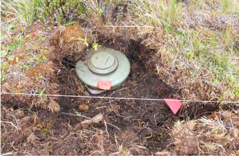
A Spanish C-3-B anti-tank mine laid in well-drained soil and protected by vegetation. Image: Fenix Insight Ltd.
