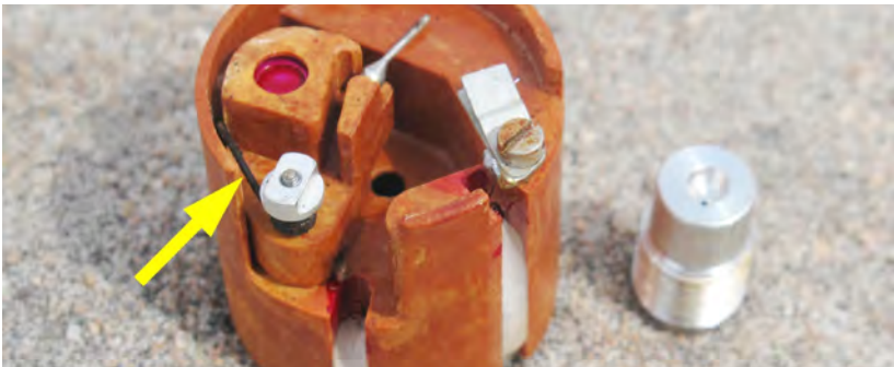
This fuze is from the Russian PTAB-2.5M submunition, which is found within the stockpiles of many countries. In this example, the small spring (yellow arrow) that turns the detonator rotor has failed due to corrosion. This spring is responsible for bringing the detonator into line with a booster and making an electrical connection. This tiny component is the only point of failure in the whole munition, but it is enough to prevent it from operating. Image: Fenix Insight Ltd.
