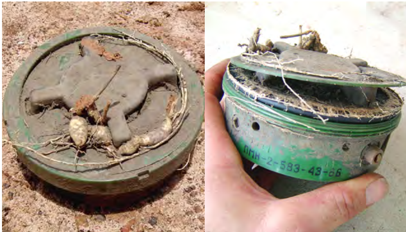
A Russian PMN-2 anti-personnel mine recovered from northern Cambodia in 2009. Small roots have spread into the small gaps and joins around the pressure plate. Disassembly of the PMN-2 mine shows that the root structure has penetrated the mine casing, levering components apart and allowing water to enter. Images: Fenix Insight Ltd.
