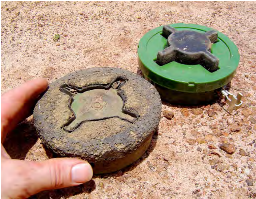
Russian PMN-2 anti-personnel mines recovered from different minefields in northern Cambodia in 2009. The mine in the foreground has been severely damaged by fire, which has burned away the cruciform pressure plate and allowed water to enter the mine. The explosive components are undamaged but, ironically, the loss of the pressure plate means that this mine could no longer function as designed. Image: Fenix Insight Ltd.
