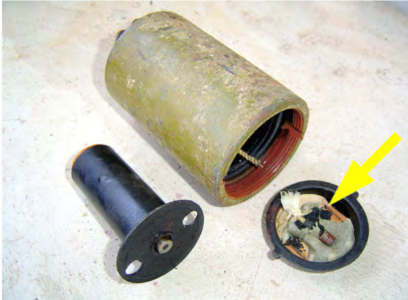
A Russian OZM-4 bounding mine, recovered from storage in Cambodia. The black powder and igniter (arrow) are still in good condition after 50 years. However, both are vulnerable to water and will fail to function if they are damp. In such a case, the initiation train will be broken and the mine will fail to operate.
