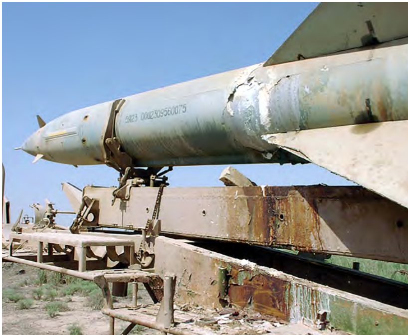
An SA-2 missile in Iraq following the war. Liquid fuel and oxidant from the rocket motor is leaking and contaminating the ground. Image: Fenix Insight Ltd.
