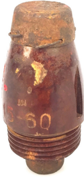
The Russian M-6 is a relatively simple mortar fuze, which incorporates an arming and impact initiation mechanism. Image left: Dutch Defence Expertise Center EOD. Image right: Fenix Insight Ltd.
