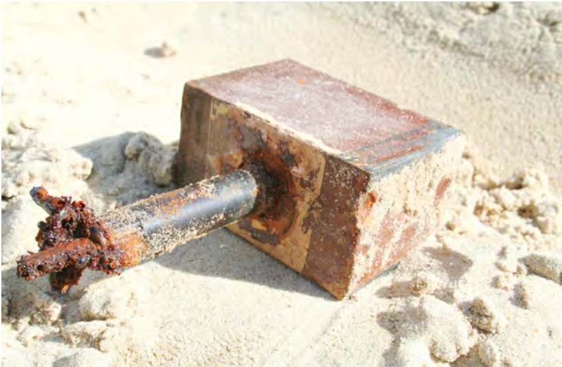
Wooden Schuminen have corroded leaving just the 200g TNT blocks in wax paper and the ZZ-42 fuzes. Note the bakelite fuze body is still in remarkably good condition but the steel striker and retaining pin have corroded. TNT has a relatively low solubility, as shown by the relative resilience of these charges, albeit these have not been subjected to prolonged saturation in salt water. Images: Martin Jebens, Danish Coastal Authority.
