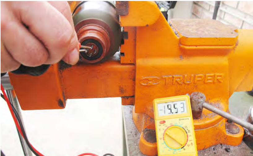
During the demilitarisation of these missiles a number of SA-7 batteries dating from the 1970s were activated and then tested; all operated correctly. This test shows a Russian 9B17 battery clamped into a vice and activated, producing more than 19 Volts, as it was originally designed to do. Image: Fenix Insight Ltd.
