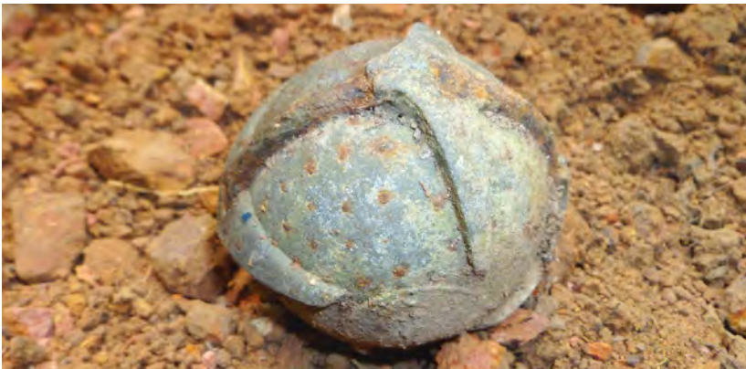
A BLU-26 explosive submunition found in Lao PDR. The steel alloy components can be seen by the difference in corrosion around the clamp ring join of the submunition and the ball bearing fragmentation beneath the main aluminium outer casing. The outer casing has an aluminium oxide layer that corrodes slower than steel alloy. This item has been on the floor of a primary jungle for over four decades, albeit on high ground with good drainage. While it is certainly weathered, the resilience of the casing is nevertheless evident. Image: Roly Evans.
