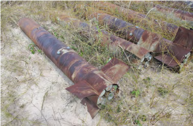
Russian S-24B rockets in a depot in Mozambique in 2014. At some point, fire has swept through the vegetation, burning the paint from the upper surfaces but failing to initiate the motors, also leaving the paint on the underside relatively unscathed.
