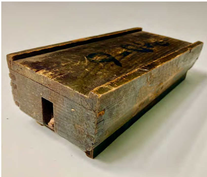
The Russian PMD-6 box mine, as it appears intact. The PMD-6 has a wooden case that was judged to be adequate for its expected short service life. It was never intended or expected to remain functional for years. Image: GICHD.
