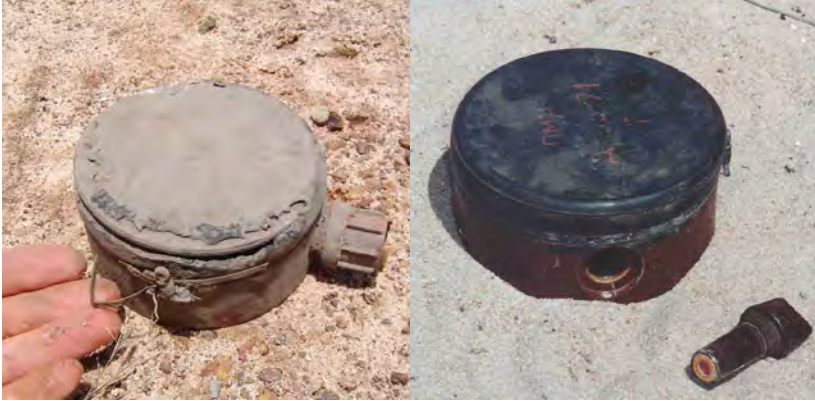
Left: A PMN mine recovered in Cambodia. The hot wet climate has caused the rubber cover to perish and the securing band to rust through. Right: A PMN of a similar age in Afghanistan has been well-preserved, with little deterioration of the rubber cover or securing band. Images: Fenix Insight Ltd.
