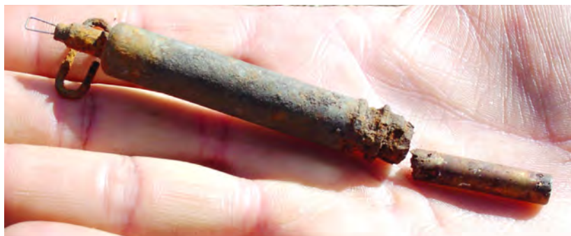
A Russian MUV-2 fuze from a PMD-6 anti-personnel mine recovered in Cambodia, 2010. The upper hollow section of the aluminium detonator capsule has corroded away, separating the explosive from the fuze. Since the mine was buried, this gap was then filled with earth and probably would have prevented the fuze from functioning. Image: Fenix Insight Ltd.
