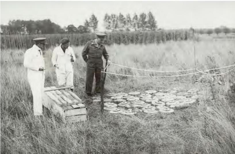
Inspecting Tellermine-42s removed from a "low lying meadow". While rusting was observed in this environment after 12 months, metal cased Tellermine were still deemed 100% effective after 18 months. Image: NIOD Institute
