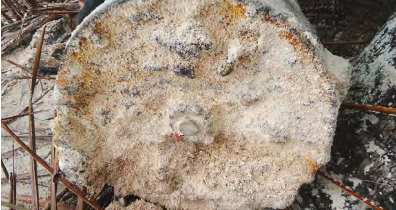
The combination of abrasive sand and salt water has accelerated the corrosion of the casing, which has partly disintegrated, leaving the explosive filling exposed. Image: Len Austin.
