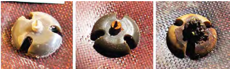
Firing pins recovered from United States M14 anti-personnel mines in Jordan during the early 2000s. The pin on the left is virtually as-new, but the pins in the centre and right have become shorter and blunter. These are unlikely to initiate the mine's stab-sensitive detonator. Corroded firing pins will also make the mine even harder to detect.
