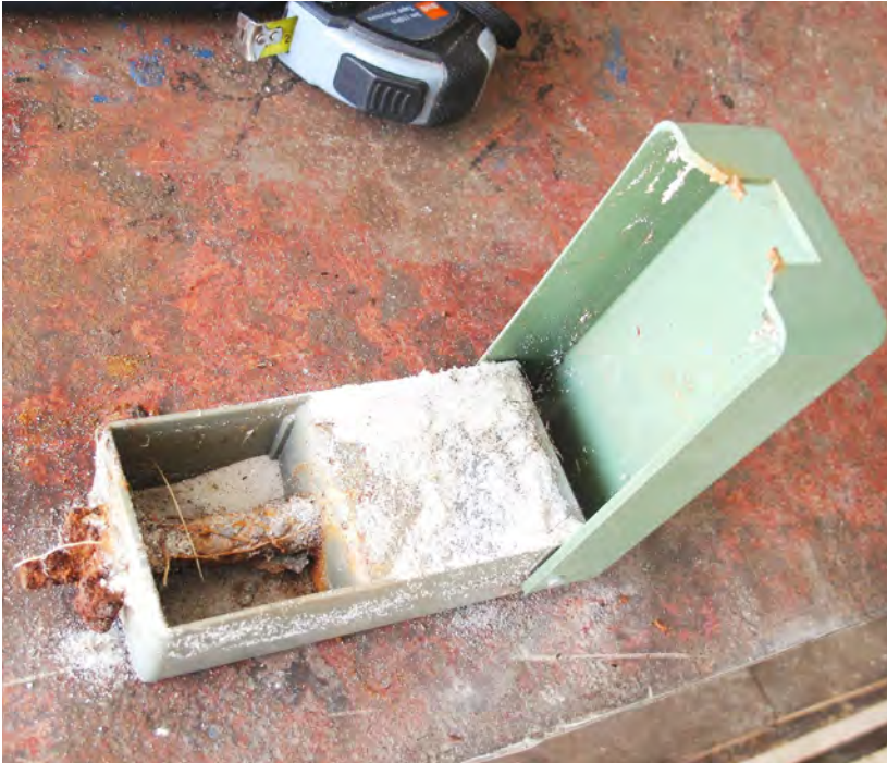
An Israeli No 4 anti-personnel mine in the Falkland Islands/Malvinas, recovered from a coastal minefield near Port Stanley in 2019. Water often carries fine particles, such as sand, which have an abrasive effect and can fill voids within the fuze mechanism, blocking its action. The No.9 fuze igniter seen here is heavily corroded and no longer functional although it still presents an explosive hazard. Image: Fenix Insight Ltd.
