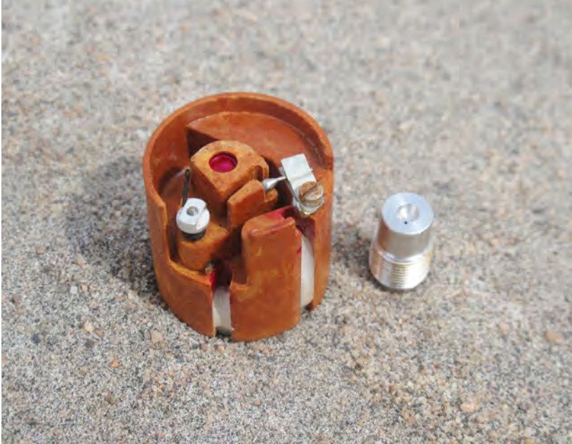
A corroded and broken detonator rotor spring in the fuze of a PTAB-2.5M submunition. Here, the fuze is seen armed, with the rotor central. However, the absence of the spring means that the rotor can now move by gravity or turning moment. Once the arming action has freed the rotor, it is a question of chance whether it remains out of line or falls into line. The orientation of the fuze is not visible from the outside, nor is it possible to see the position of the rotor. This means that it may alternate between being armed and unarmed as it is moved. Corrosion of the rotor spring has made this item more dangerous. Image: Fenix Insight Ltd.
