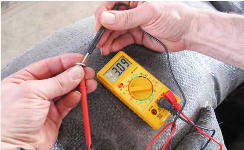
The batteries were manufactured in 1996. Testing showed that the batteries still retained full charge, around 25 years after they were manufactured. Image: Fenix Insight Ltd.
