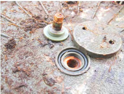
Examination shows that the loose plug allowed water to enter the casing, saturating the detonator over time.
