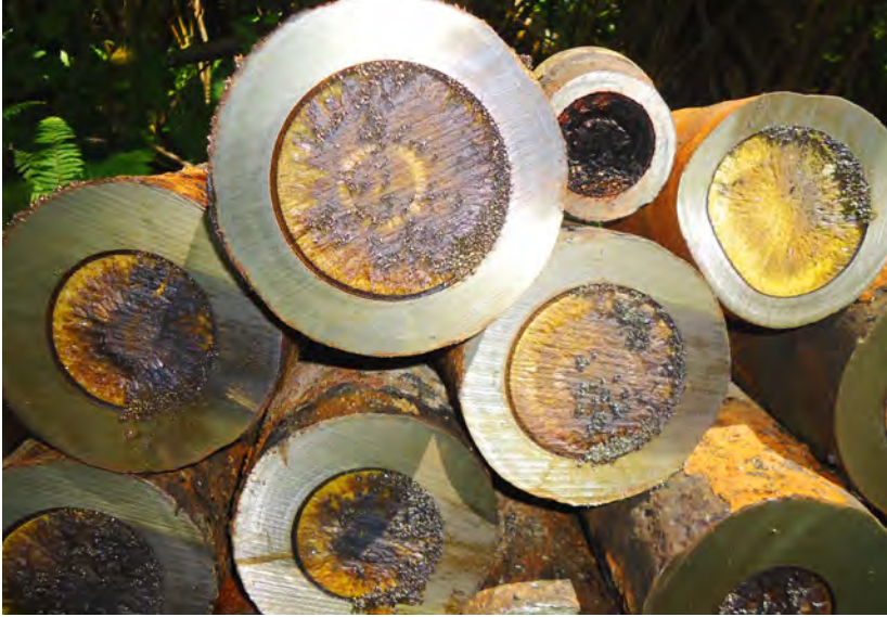
Cuts through 75mm and 15cm projectiles show that, despite the external corrosion, there is still plenty of unaffected steel. The yellow explosive filling is based on TNT, which darkens to a brown colour when it is exposed to light. Image: Len Austin.
