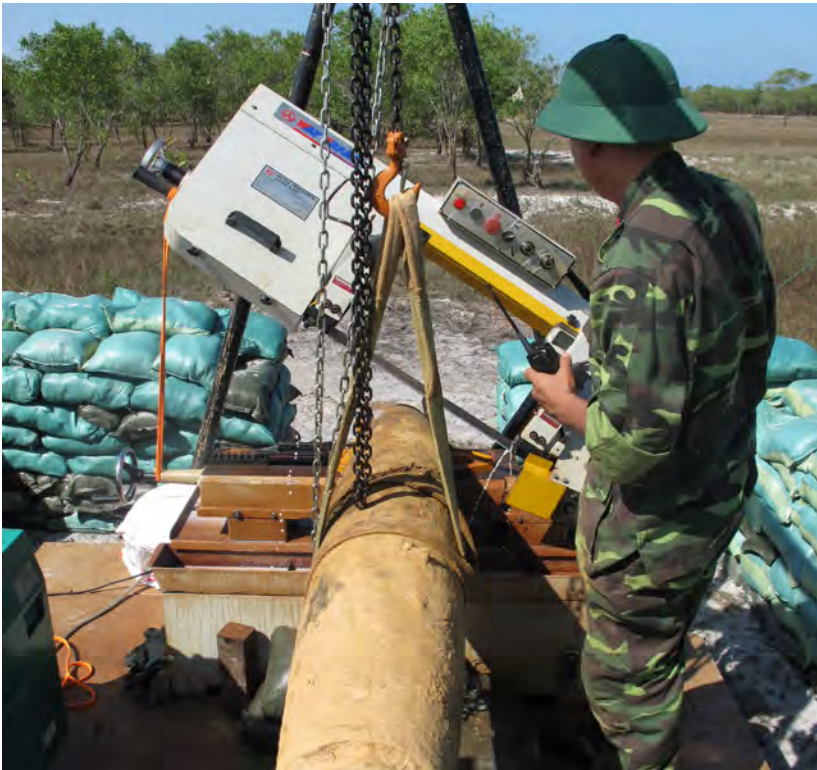
A portable cutting deck, operated by the Golden West Humanitarian Foundation in Vietnam. Access into thick-cased munitions, such as mortar bombs, projectiles and air-dropped bombs, can be achieved using commercial bandsaws, which are adapted for remote operation and observation. This is a specialist task but, performed properly, allows even the largest ordnance to be sectioned and examined internally. In this instance a Vietnamese soldier from Technology Centre for Bomb and Mine Disposal Engineering Command (BOMICEN) sets up a cut on a Mk-82 General Purpose Bomb. Image: Fenix insight Ltd.
