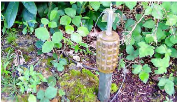
Contrary to popular belief, most tripwires are made from iron or steel, with little or no protection. Tripwires used with mines like this Chinese Type 59, laid in Cambodia more than 40 years ago, rusted away many years ago. Image: Fenix Insight Ltd.
