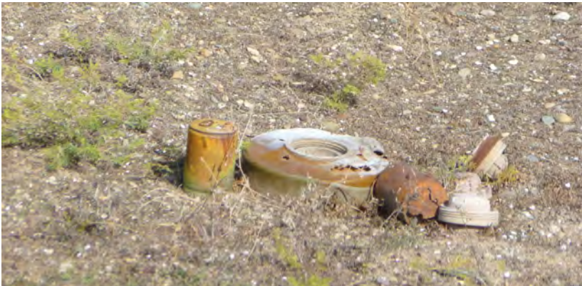
Various mines in the same environment show different ageing characteristics. The relatively thin plastic cased TM-62P3 anti-vehicle mine shows rupture of the casing, possibly accentuated by the effect of prolonged exposure to ultraviolet (UV) sunlight. The thicker cased MVP and MVCH mine fuzes seen on the right are more resilient, albeit their colour has bleached in the sun. The OZM-72 bounding fragmentation mine on the left shows discolouration of the protective paint but has broadly withstood the ageing process well. Image: Roly Evans.
