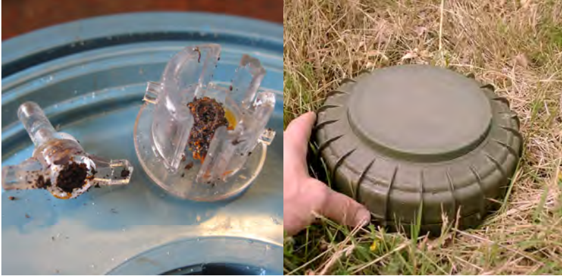
Externally, SB-81 anti-tank mines recovered from coastal areas of the Falkland Islands/Malvinas in 2019 looked similar to those used inland, since there was very little deterioration of the casing. Usually an intact glass reinforced polycarbonate casing would imply functioning internal components. However in this instance some water ingress into the casing has taken place. The presence of salt water in mines from coastal areas has had a significant corrosive effect on the metallic fuze components. The polycarbonate plastic fuze components have proved more resilient. Images: Fenix Insight Ltd.
