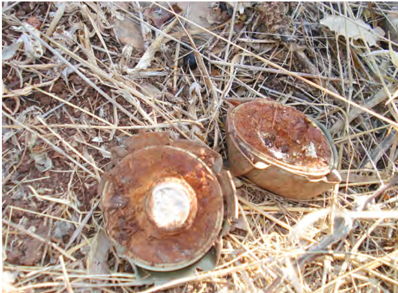
A BLU-63 submunition that has split apart on impact, exposing the cyclotol explosive fill and aluminium encased M219E1 fuze to the elements. This item will age far quicker than one that was undamaged on impact. Image: Roly Evans
