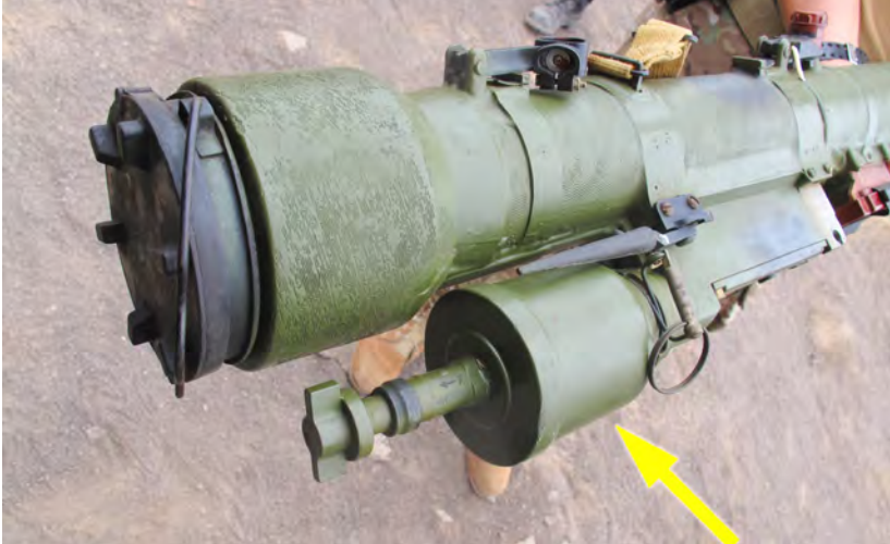
Shoulder fired air-defence systems such as the Russian SA-7, SA-14, SA-16 and SA-18 missiles use thermal batteries. These are fitted to the launcher and activated by twisting a key at the end of the battery assembly. Once heated up, the battery provides power for a few minutes before it cools and expires permanently. Image: Fenix Insight Ltd.
