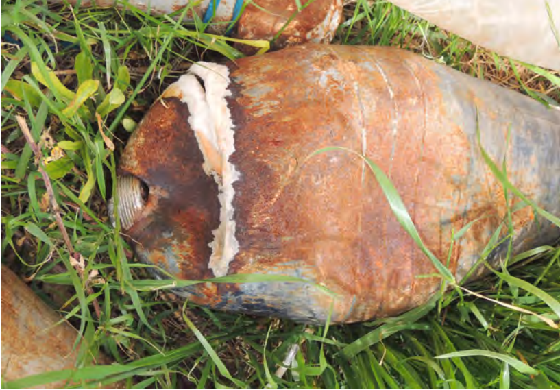
Ammonium nitrate HME exudation from a 220mm improvised mortar, April 2015, Kobane, Syria. The mortar contained knotted detonation cord to act as a booster. Detonation cord is susceptible to hygroscopic action. Image: Bob Gravett.
