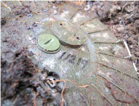
While the mine's glass reinforced polycarbonate casing is extremely resilient, the mine's detonator plug was not properly tightened when the mine was laid.
