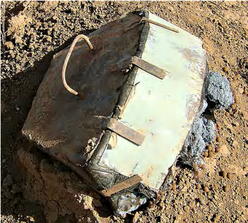
Improvised explosives such as ammonium nitrate and aluminium mixtures, pictured here in an IED found in Iraq, are far more vulnerable to deterioration than military high explosive. Unlike factory-made munitions, IEDs frequently fail because of the degradation of their main charges. Image: Bob Gravett.
