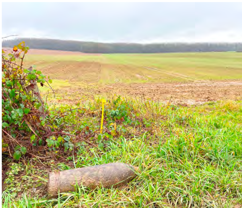
A British 6-inch artillery projectile with the copper driving band removed found close to the old German front line of August 1916, near Guillemont, Somme, France in December 2021. Note that the projectile is in remarkably good condition. Explosive ordnance that is made to withstand extreme forces on firing, and whose casing is designed to produce fragmentation, are resilient, especially in clay soils with higher pH values, and pose a long term hazard. Image: Quentin Naylor.
