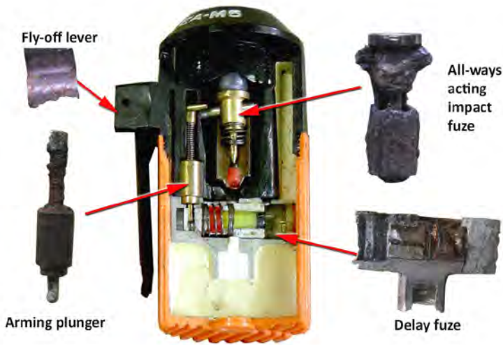
The Spanish M-5 is a complex hand grenade incorporating both delay and impact fuzes. This image shows a section through a new grenade, along with aged components from an example recovered in the Falkland Islands/Malvinas in 2015, 33 years after the war. The multiple points of failure among both mechanical and energetic components meant that the risk from the aged grenade was minimal. Image: Fenix Insight Ltd.
