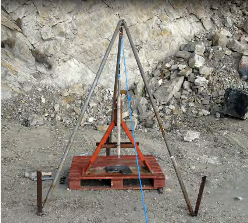
An improvised explosive test rig in the Falkland Islands/Malvinas. During this operation, landmine fuzes were first separated from their main charges, substantially reducing the explosive hazard, and therefore the safety distance. Using remote operation and observation, a weight was dropped onto the fuze to see if it would function. The rig was sufficiently strong to withstand the detonation of the small amounts of explosive within the fuze. Image: Fenix Insight Ltd.
