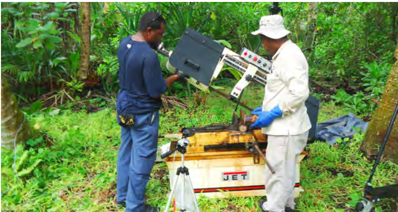
A portable cutting deck, based on a commercial bandsaw, conducting exploitation of Japanese 75mm Type 94 HE projectiles. While not a conventional ammunition process facility, mobile cutting stations can still conduct exploitation safely by effectively controlling the surrounding area as a range. All cuts are conducted remotely. The TNT fill is ultimately disposed of by open burning. Image: Len Austin.
