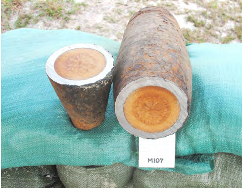
A Vietnam-era 155mm United States M107 projectile, recovered in Quang Tri province and cut open for analysis in 2018. The Composition B filling, which is a mixture of RDX and TNT, shows virtually no sign of deterioration over the 50 years or so since it was manufactured. Most of the military high explosives used in main ammunition fillings are extremely stable and resilient even when the casing has deteriorated. In this case the casing has protected the main explosive fill remarkably well.
