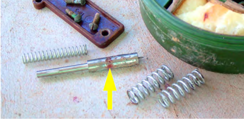
The springs in this Russian PMN-2, also recovered from Cambodia in 2014, are in good condition; however, the plating on the striker has been lifted and bulged by corrosion (yellow arrow). Because of the fine tolerances in the fuze, this small dimensional change is sufficient to seize the striker into place and prevent the mine from operating. Image: Fenix Insight Ltd.
