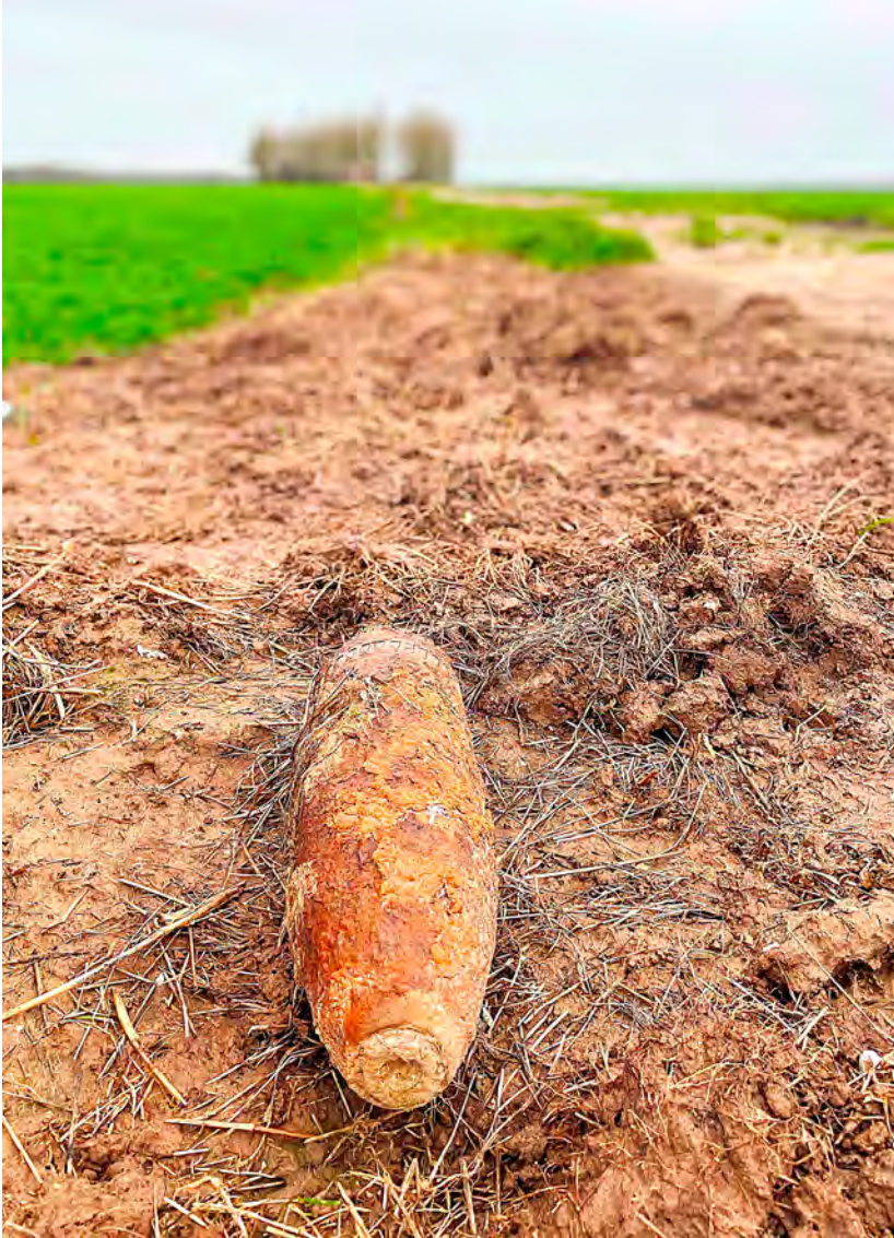
A British 4.5 inch artillery projectile near Thiepval, Somme France, January 2023. The rotating band and copper fuze adaptor for the Fuze No. 44 show how resilient copper and copper alloys can be despite prolonged exposure in the environment for over 100 years. The layer of clay soil has very likely also helped to preserve the projectile. Image: Quentin Naylor.
