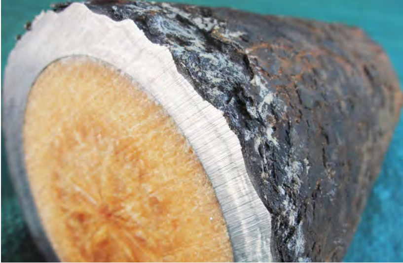
The casing of an unexploded M107 projectile, recovered around 50 years after it was used in Vietnam. A section through the projectile shows the surface is heavily corroded, although the steel beneath is in remarkably good condition. Under some circumstances, a superficial iron oxide rust layer may provide protection that slows down the corrosion process. Image: Fenix Insight Ltd.
