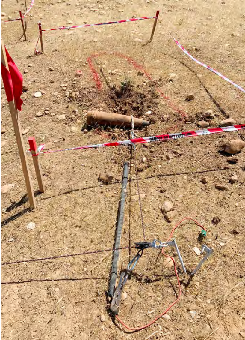
A semi-remote pull on a high explosive 130mm artillery projectile employed as a main charge in an IED, Tel Kaif district, Mosul, May 2022. Use of ERW typically results in IEDs with a far more resilient main charge than those employing improvised explosive mixtures. Image: Daniel Davids.
