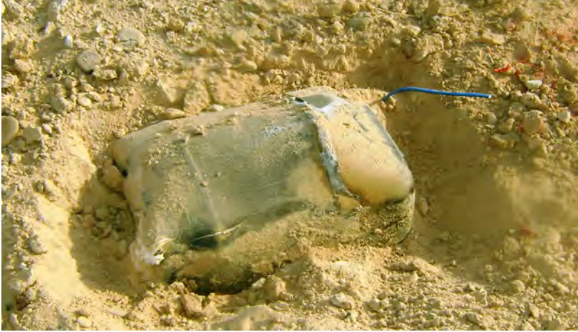
An expanded aluminized ammonium nitrate charge in a 20 litre plastic container, Jalawla, Kurdistan Region of Iraq, August 2016. Expanded charges would routinely split plastic casings. Image: Bob Gravett.
