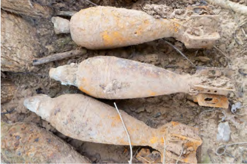
Weathered AXO gathered by local farmers. Note that corrosion of the fuzes is more advanced than on the mortar bodies. Image: Roly Evans.
