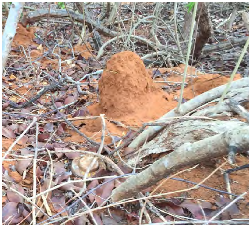
A P4Mk2 anti-personnel mine on the jungle floor in Sri-Lanka. The plastic casing is relatively resilient. The sandy soil drains quickly. Many mines found here were still viable. Image: Roly Evans.
