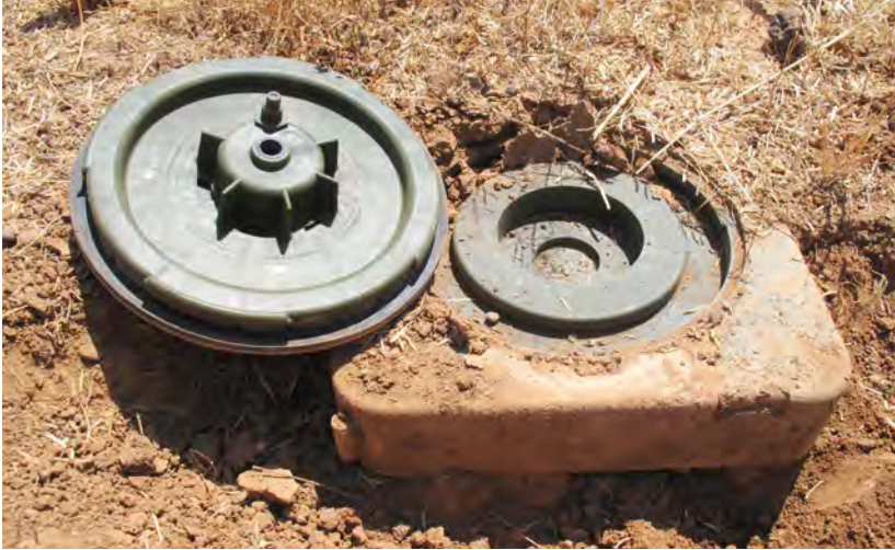
A United States M19 anti-tank mine in Jordan. The mine is fully functional and shows few signs of deterioration, despite having been buried for around 40 years. The relatively thick plastic and rubber seals around the threads protect the internal components of the mine. Many M19s cleared in Afghanistan have also been found in good condition. While more susceptible to UV damage if exposed to prolonged sunlight, buried mines with thick plastic casings can be very resilient, possibly as resilient as steel cased ERW in certain circumstances. Image: Fenix Insight Ltd.
