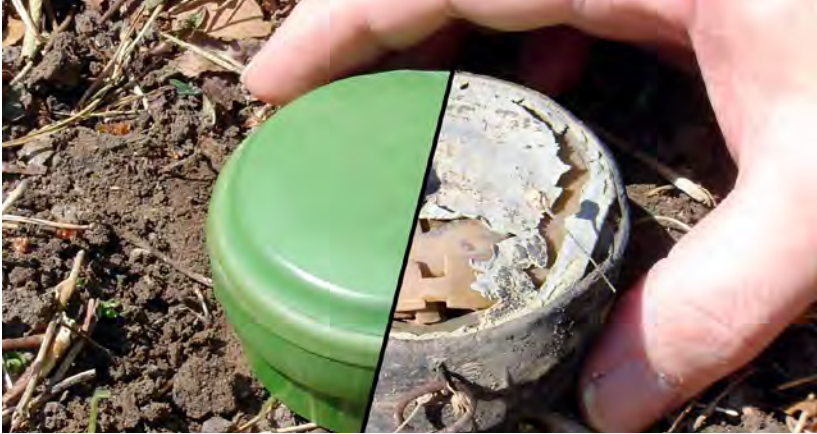
A composite image contrasting the appearance of a new Chinese Type 72 anti-personnel mine (to the left) with its appearance after years of exposure to sunlight in Cambodia. The green cover is made from thin rubber, which becomes grey and perishes, exposing the buff-coloured pressure plate beneath. The result is that the aged mine looks nothing like it did when new, making it difficult to recognise.
