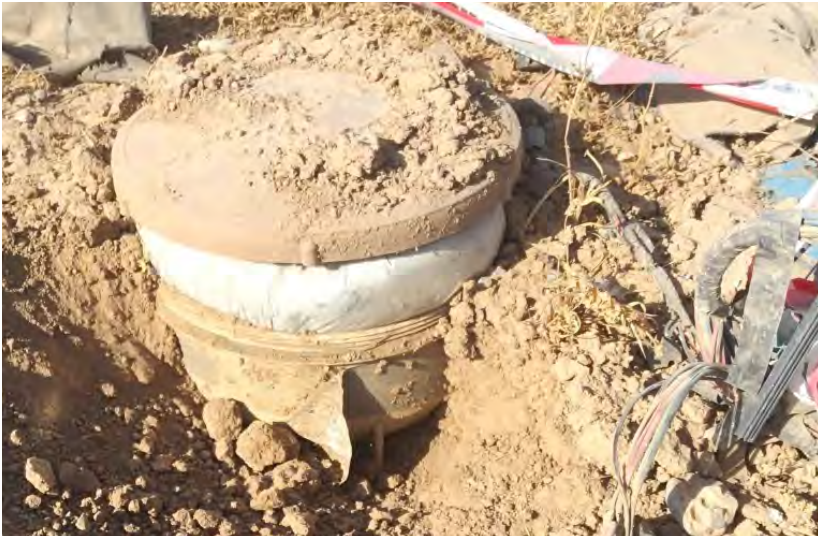
Image top shows a heavily corroded improvised mechanical fuze used in the mechanical version of the VS-500. Image bottom shows expansion of the aluminized ammonium nitrate main charge in an electrically initiated VS-500. Both images: FSD.
