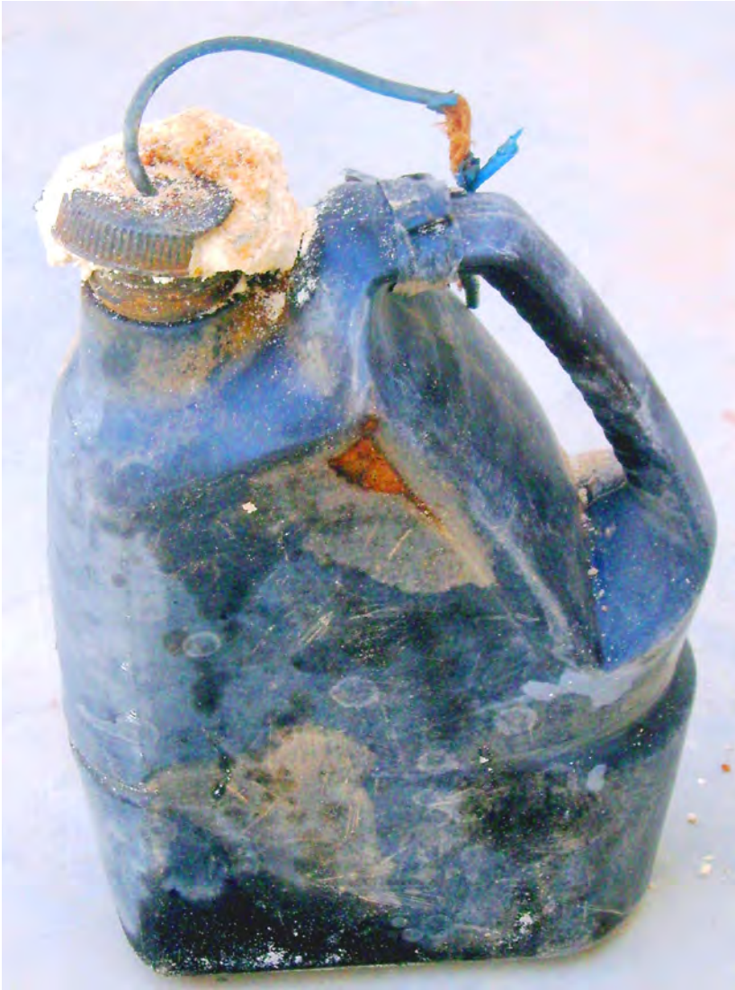
Ammonium Nitrate exudation from the neck of a 5ltr Improvised Plastic IED, Khan Village, Kobane, Syria, July 2016. This main charge was probably emplaced at some point in 2014. It is likely a result of phase changes due to temperature causing expansion and rupturing of the casing at the screw thread. The booster charge was fashioned from knotted detonation cord, which is also prone to hygroscopic action if water breaches the casing. Image: Bob Gravett.
