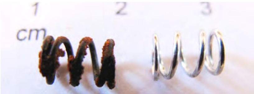
Springs from P4B minimum metal anti-personnel mines, one corroded, another not. The corroded spring's conductivity will reduce making the mine harder to detect. For minimum metal mines, corrosion of the only metallic components makes them even harder to detect. Image: Fenix Insight Ltd.
