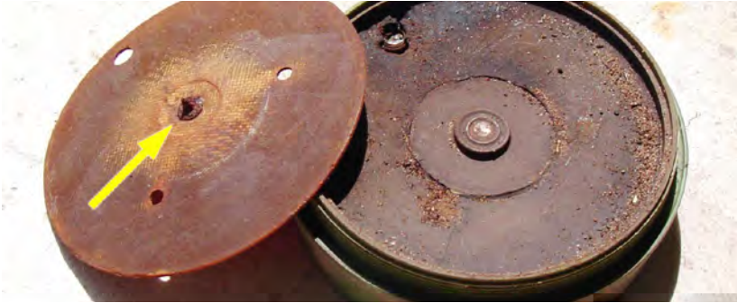
The Chinese Type 72 anti-personnel mine has a firing pin (arrow) weighing just 0.12g, which makes it barely detectable. Any significant loss of metallic mass, as the pin rusts, may take it below the detectability threshold, even though the pin may still be long enough to fire the stab-sensitive igniter. This may have been the case with some of the mines examined in Cambodia in 2015. Image: Fenix Insight Ltd.
