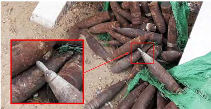
Russian 30mm cannon ammunition in Afghanistan, 2020. Some of the A-670M fuzes have lost their windshields, allowing water to penetrate the fuze body. Image: The HALO Trust.
