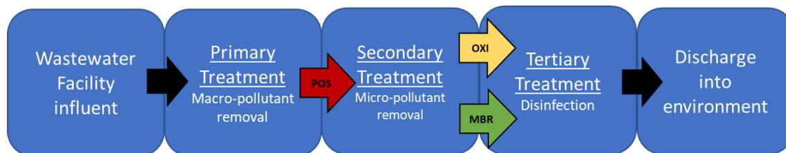
*Note.* Includes primary treatment that removes macro-pollutants, secondary treatment for nutrient and micro-pollutant removal, and tertiary treatment for disinfection. After treatment the water is discharged into the environment. Colored arrows represent treatments in this study primary effluent (POS) and two different secondary treatments oxidation ditch effluent (OXI) and membrane bioreactor (MBR).
