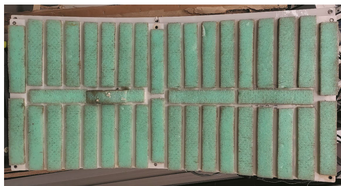
Figure 6. After-market modification of a flexible solar PV module by taping PE foam on the back layer of the modules using polyurethane marine sealant
