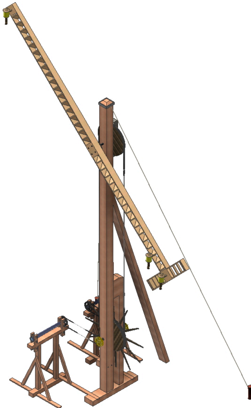
Figure 22. Optical telegraph assembled with all its elements.
