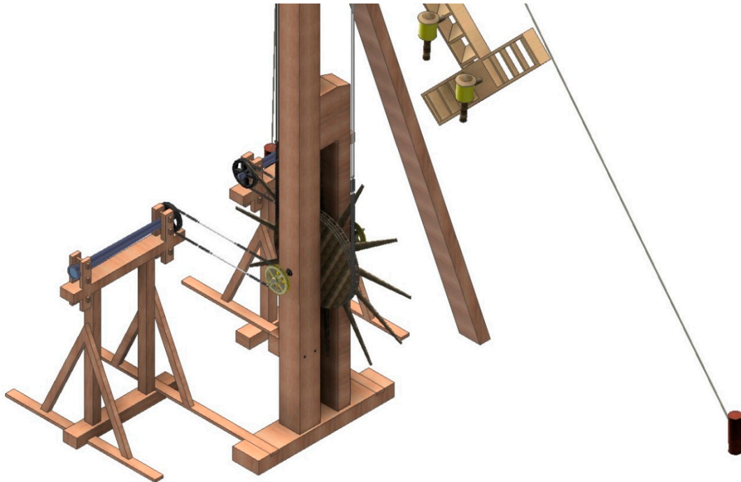
Figure 10. Detail of the position of the winch on the mast frame.
