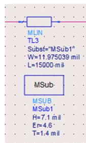
Figure 41: MLIN Transmission Line.
