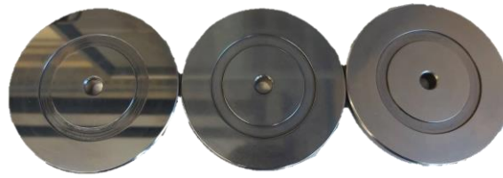
Figure 2.16 Steel discs with different roughness for Stribeck Curve measurements
