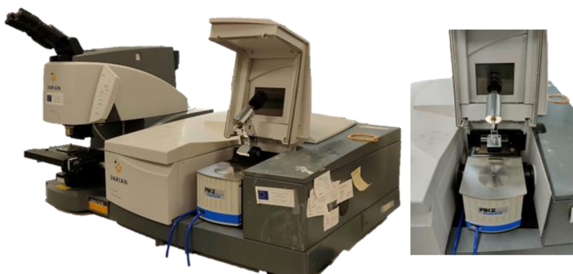
Figure 2.5 Fourier transform infrared spectrometer: FTIR VARIAN 670-IR (RIAIDT of the USC)
