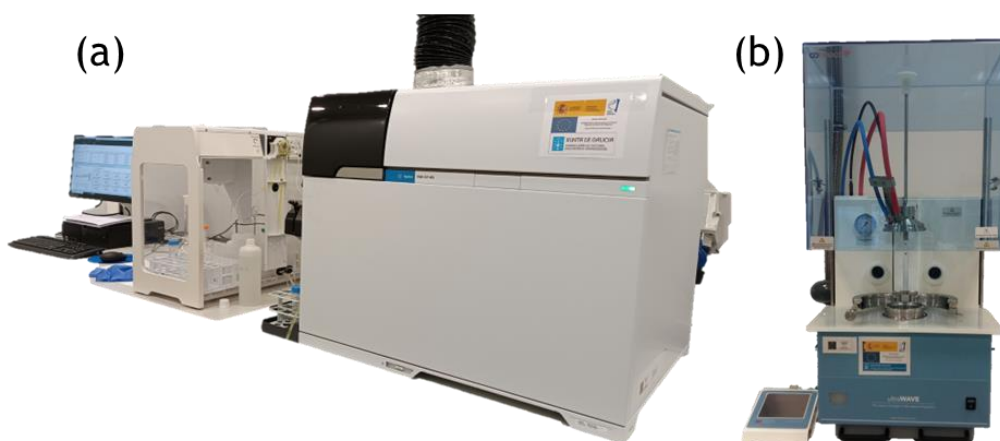
Figure 2.9 Equipment for elemental analysis (RIADT of the USC): (a) Inductively coupled plasma mass spectrometer Agilent 7900x; (b) Milestone ultraWAVE3 microwave digestion system
