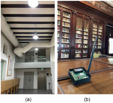
Fig. 12. Cultural center 'La Nau': (a) roof made of wood; (b) LoRa MC end-node sensor measuring values in the library section of the building.
