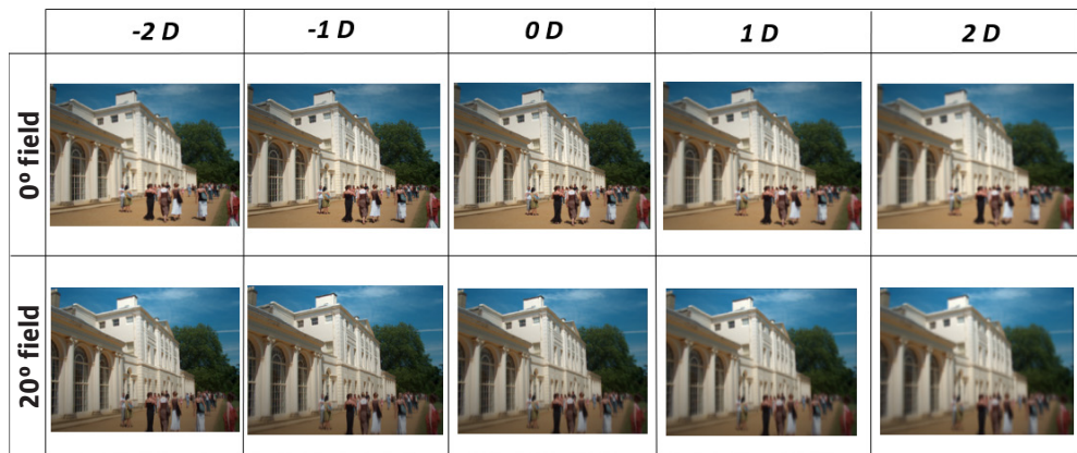
FIGURE 12. Image simulation through focus and different fields. Pupil diameter is 3 mm
