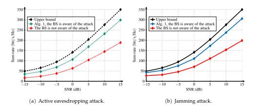
Figure 2: Sum rate by considering K = 10 users, M = 400 antennas at the BS, L = 20 pilot symbols, and different strategies to configure the precoders and power allocation.
