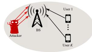
Figure 1: Pilot attack model in a multi-user (K users) uplink MaMIMO system.
