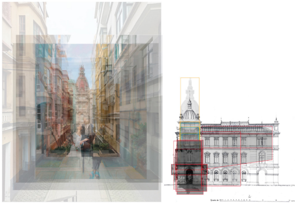
Figure 3: [left] Overlapping of photographs located at two distances from the town hall on the same street, drawing and editing, Ledo Romay, 2021; [right] Overlapping of cropped photographs on the east elevation of the A Coruña City Hall, where the colors of the frames identify the distance of each photograph, Ledo Romay, 2021.
