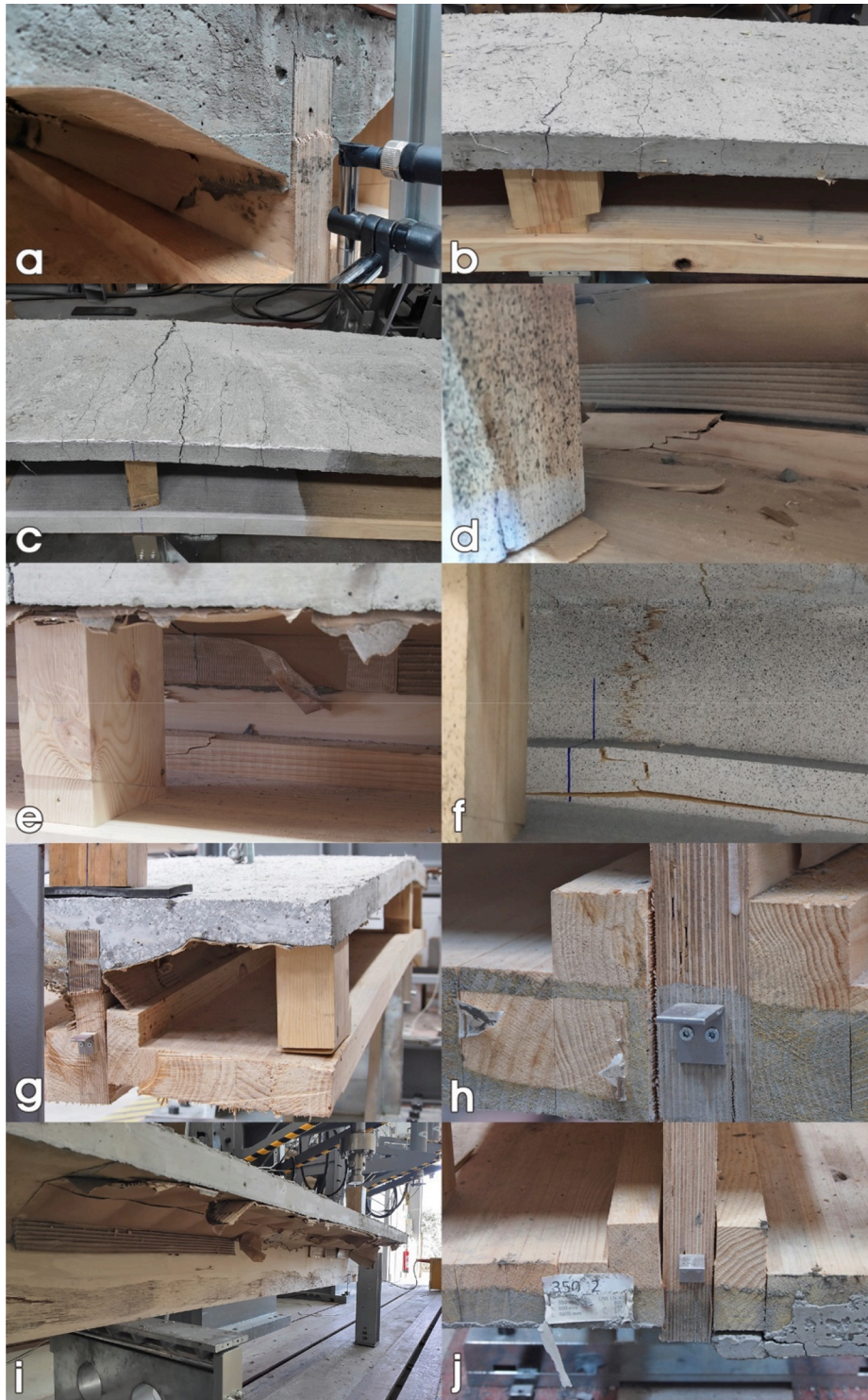
Fig. 6. Failure modes. Samples: 250.1-X (a, b, d); 250.2-X(h); 250.1-Y(g); 300.1-X(i); 300.2-X(e); 300.2-Y(b, f); 350.2-X(j). Note: images e, g, i show the remains of cardboard corresponding to the vaults used as lightening elements and that were partially removed to observe the damage to the wood
