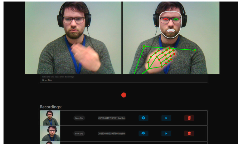
Figure 6. Screenshot of the interface of the gesture video recording application. The video stream on the right-side overlaps with visual elements representing the recognized skeletal key-points (red dots) and the corresponding connections between them (green lines).
