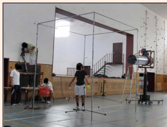
Figure 1. Three-dimensional reference system for the analysis of the toss ball in three points ( x, y, z ): Initial, Peak point and impact point of the players.
