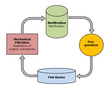
Figure 9: Schematic illustration of a closed recirculation aquaculture system
