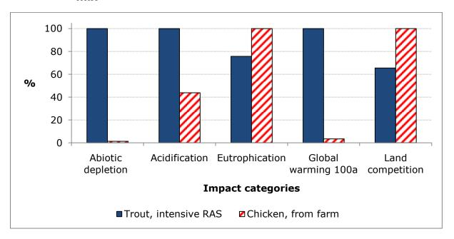
Figure 11: Comparative LCA of trout produced in intensive RAS and chicken produced in farms using alternative energy sources
