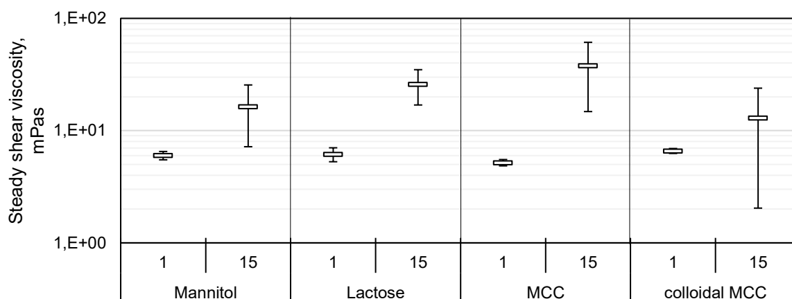
Figure 6-7: Steady shear viscosity of 2% dispersions of fillers in SNF after 1 min (1) and 15 min (15) resting time at a shear rate of 1 \text{ s}^{-1} . n=3 ; error bars show standard deviation.
