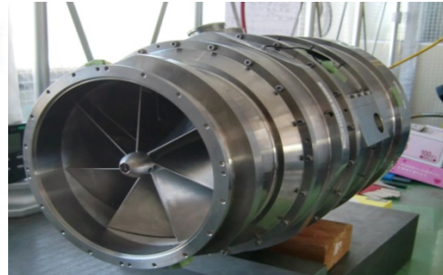
Figure 2 GG-ATR Engine developed in Muroran Institute of Technology
