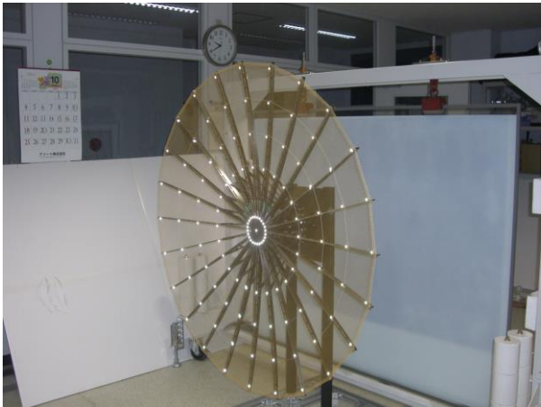
Fig. 7 Parabolic mesh antenna for radio wave test model for ASTRO-G satellite
