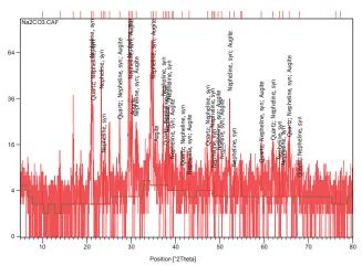
Fig. 8. X-diffraction patterns of Soda slag
