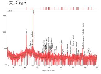
Fig. 4. X-diffraction patterns of dreg A
