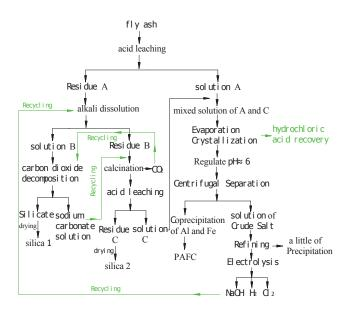
Fig. 1. The overall use technology of Fly Ash
