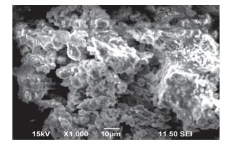
Fig. 9. SEM chart of Soda slag
