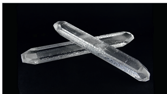
Figure 3. (a) Autoclave for growing synthetic quartz crystals (of 650 mm in total inside diameter, and 14 m in total inside height). Figures cited from Reference [9]. (b) Grown Y-bar synthetic quartz crystals.
