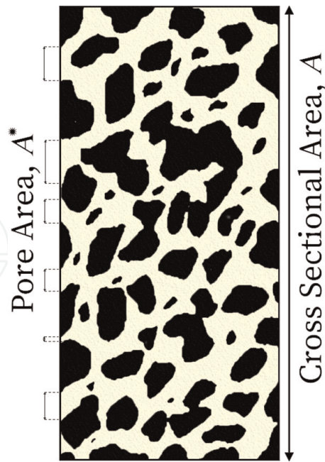
Figure 8. Open pore area at a given cross-section of a porous material: Rearrangement from Culot, Olson [181].
