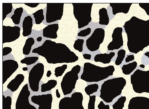
Legend for Figure 3: Grey box: Interstitial water-filled volume, V_w Black box: Solid grains, V_s Yellow box: Void gas-filled volume, V_a
