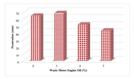
Figure 1: Penetration value of waste motor engine oil in warm mix asphalt
