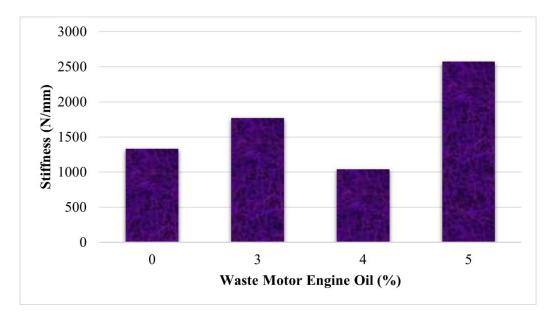
Figure 5: Stiffness of warm mix asphalt containing waste motor engine oil
