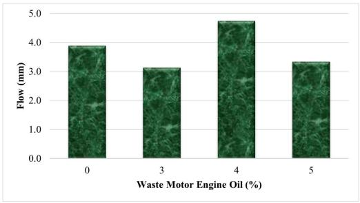
Figure 4: Flow of warm mix asphalt containing waste motor engine oil
