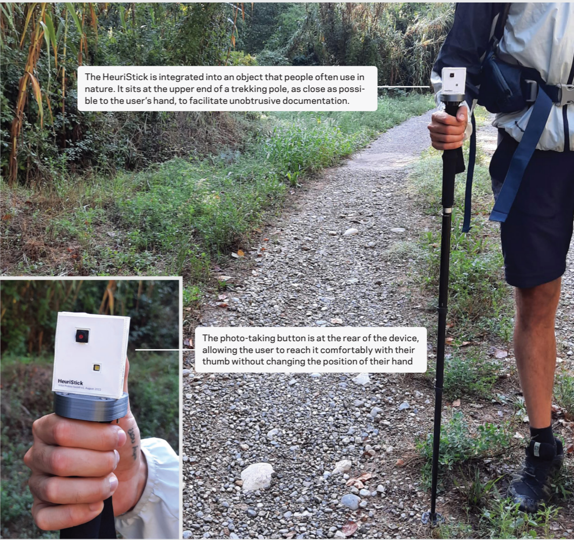
Fig. 2. The HeuriStick extends trekking poles by allowing users to rapidly document (on photo and video) spontaneous events.
