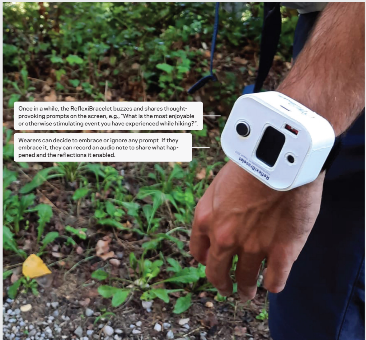
Fig. 6. Like the MemoCollar, the ReflexiBracelet enables seamless documentation through audio notes. Yet, this WP also sends thought-provoking questions to the wearer to encourage them to focus on specific aspects of their forestry experiences.
