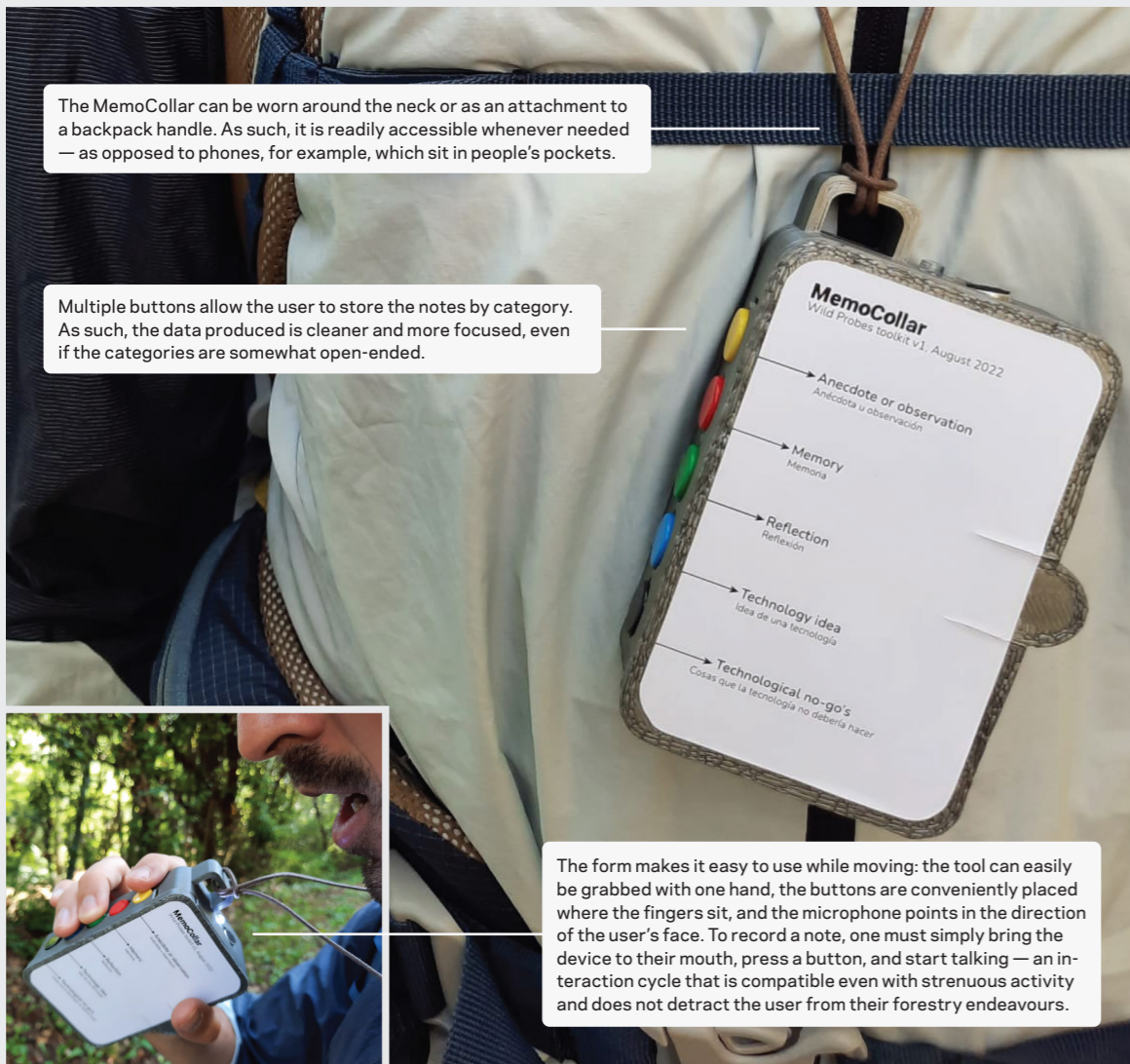
Fig. 4. The MemoCollar records voice notes so that co-designers can seamlessly store their thoughts, ideas, and observations as they engage with the forest.
