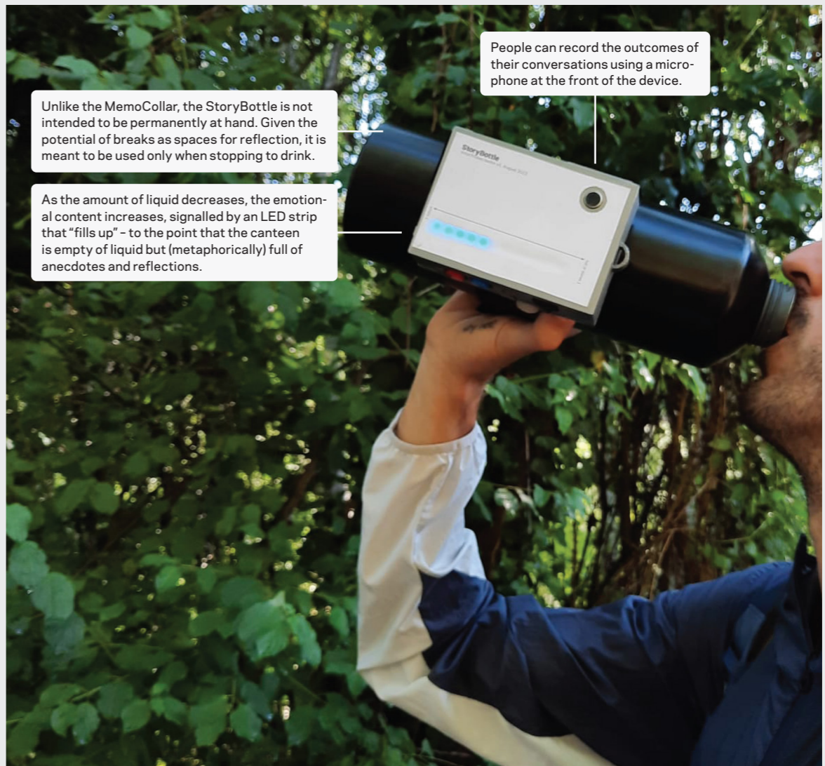
Fig. 10. The StoryBottle is an attachment to a hiking canteen that allows users to store audio notes anytime they stop to drink water: a time when discussion among hikers often takes place (Altarriba Bertran et al. 2022).
