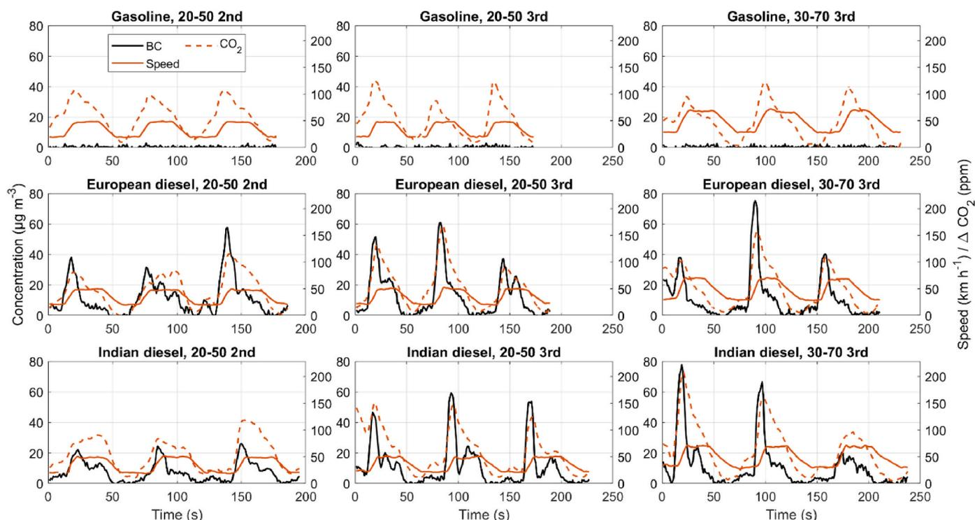
Fig. 5. Black carbon concentrations of fresh exhaust plumes of gasoline car and diesel car with two different fuels. Also the speed of test vehicle as well as increase of exhaust plume  $\Delta\text{CO}_2$  concentrations (background  $\text{CO}_2$  was subtracted) are shown.
