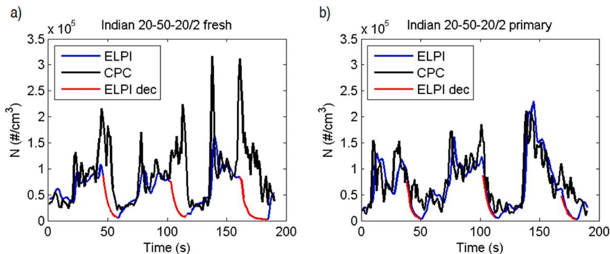
Fig. 4. Fresh (a) and primary (b) particle number concentrations for the Indian diesel during 20-50-20 cycle with 2nd gear measured by the ELPI and CPC. Also shown are the concentrations during engine braking (red color). Note that both the ELPI data and CPC data have been corrected by the same correction factor for the losses in the thermodenuder.
