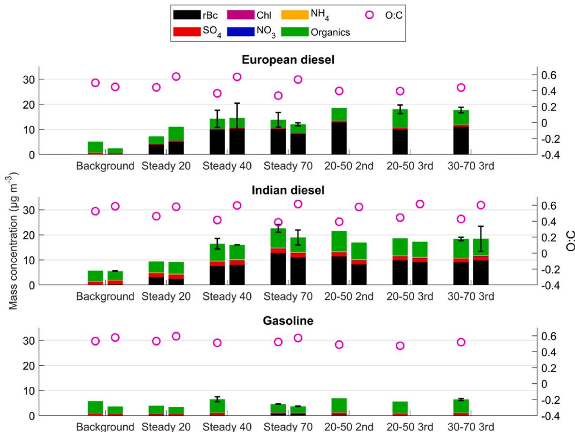
Fig. 6. Mass concentrations of the components of exhaust particles (left axis) and O:C ratio of particles (right axis). AE33 was used for the BC, other components and O:C were measured using the SP-AMS. Two bars are shown for each driving situation, left bar indicating fresh exhaust particles and the right-hand bar indicating aged exhaust particles.
