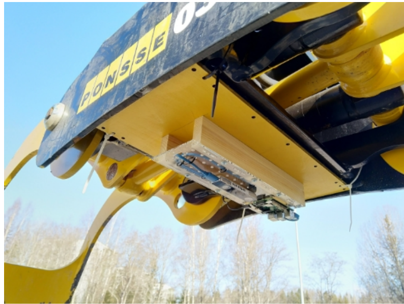
Figure 3.5. Measurement system attached to real grapple
