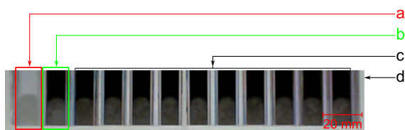
Fig. 2: Cropped frontal photograph of a representative experiment, showing a control cuvette without ink (a), a cuvette with unsonicated ink (b), ten cuvettes with sonicated ink (c), and a cuvette housing (d). The top of each cuvette comprised n -octanol, whereas the bottom comprised distilled water.
