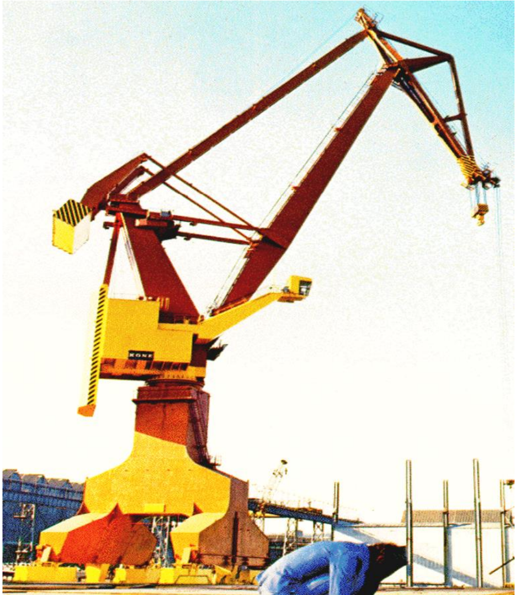
Figure 4. Articulated boom crane [2].
