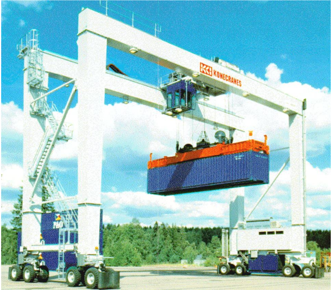
Figure 2. Rubber tired gantry crane [2].
