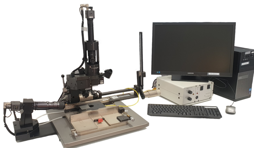
Figure 3.11. The alignment machine which was used to align and bond both layers accurately.
