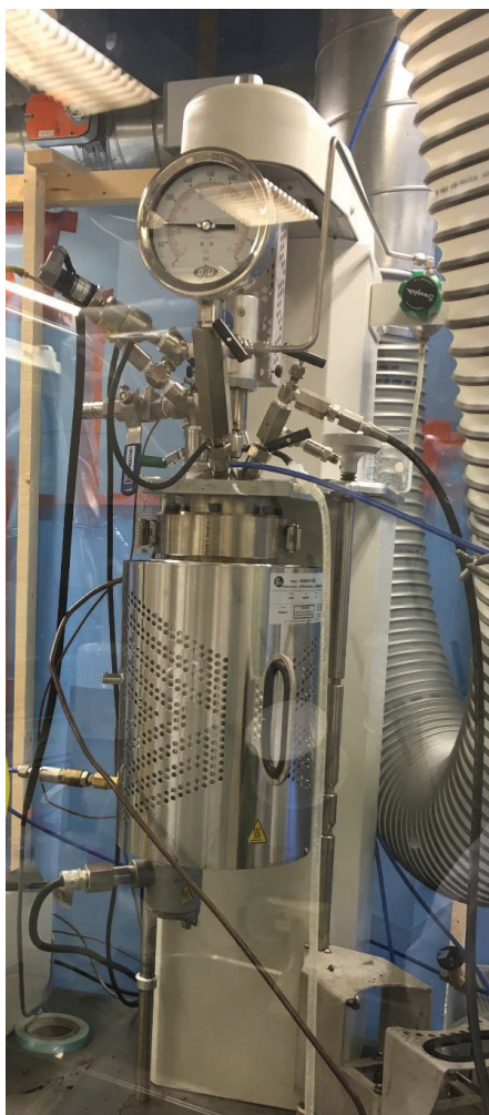
Figure S1. The HTC reactor used in the experiments was a two-liter Parr® 4500 pressure reactor with an external circulating cooling water jacket surrounding the vessel.
