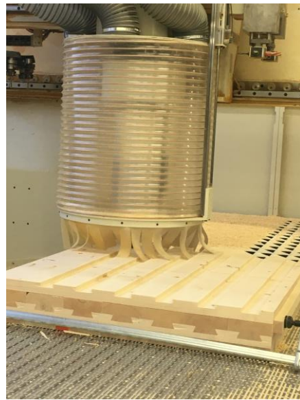
Figure 5. The manufacturing of DMWBEs at Vocational College Lapland in Kemi, Finland involved the utilization of a CNC machine equipped with a 5-axis configuration.
