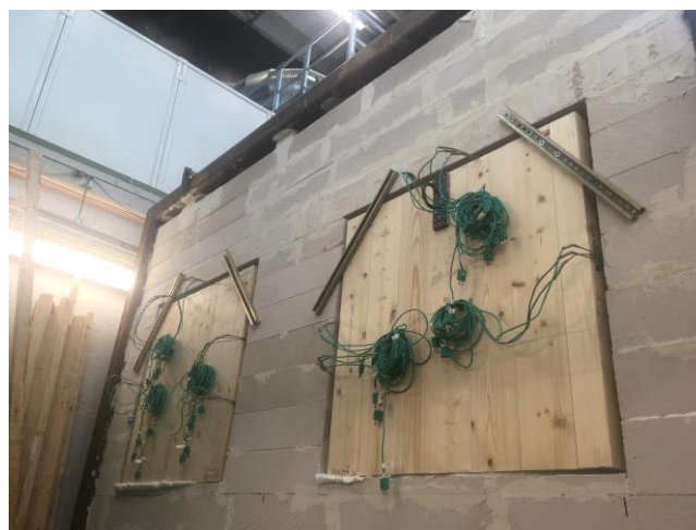
Figure 8. The specimens were affixed to a supporting structure composed of aerated concrete blocks. (Unexposed surface).
