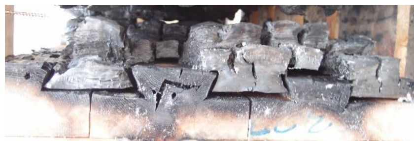
Figure 14. Remaining lamella layers and the dovetail structure of DMWBEs at the end of the test.
