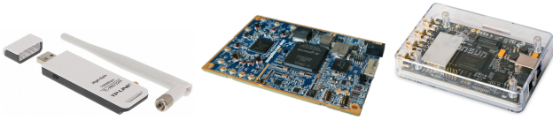
Fig. 1. Selected HW enablers for wireless network analysis (from left: TP-LINK, LimeSDR and BladeRF)
