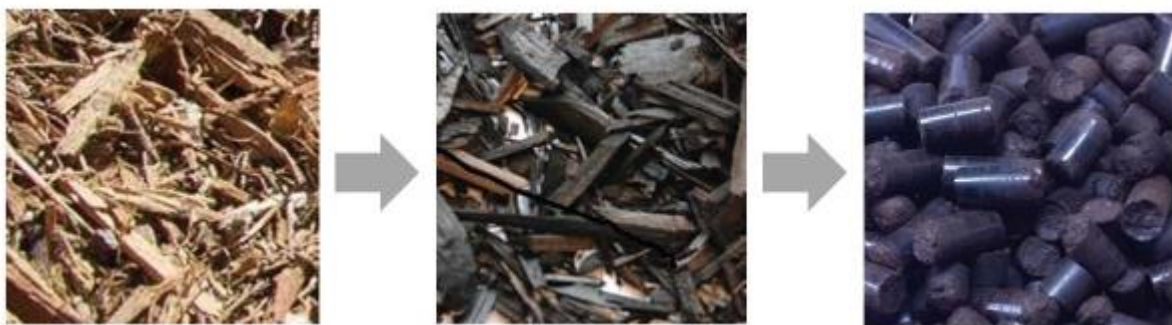
Figure 2.8 - Conversion of Raw Biomass to Torrefied Biomass to Torrefied Pellets. Retrieved from (Shah & Manandhar, 2018).
