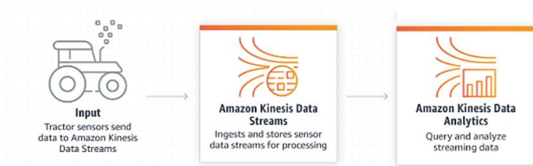
Figure 13 - Scenario using Kinesis Data Streams and Kinesis Data Analytics. Adapted from [56]
